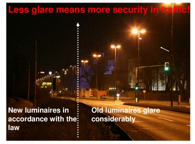
Tivolska road, during the renovation of street lighting. Old luminaires with a concave protective plastic shielding result in a lot of glare, while the glare is considerably reduced in the other half of the road where the luminaries emit 0% above the horizontal (in accordance with the Decree). All the photos: H. Mikuž and A. Mohar.
